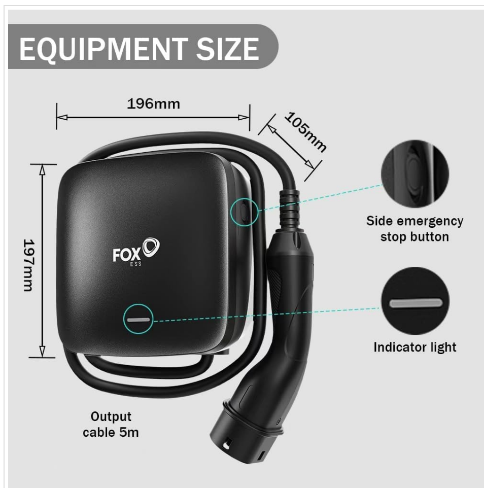
Image: Detailed dimensions of the FoxESS L07P Wallbox, including its 197mm height, 196mm width, 105mm depth, and 5m output cable. It also points out the side emergency stop button and indicator light.
