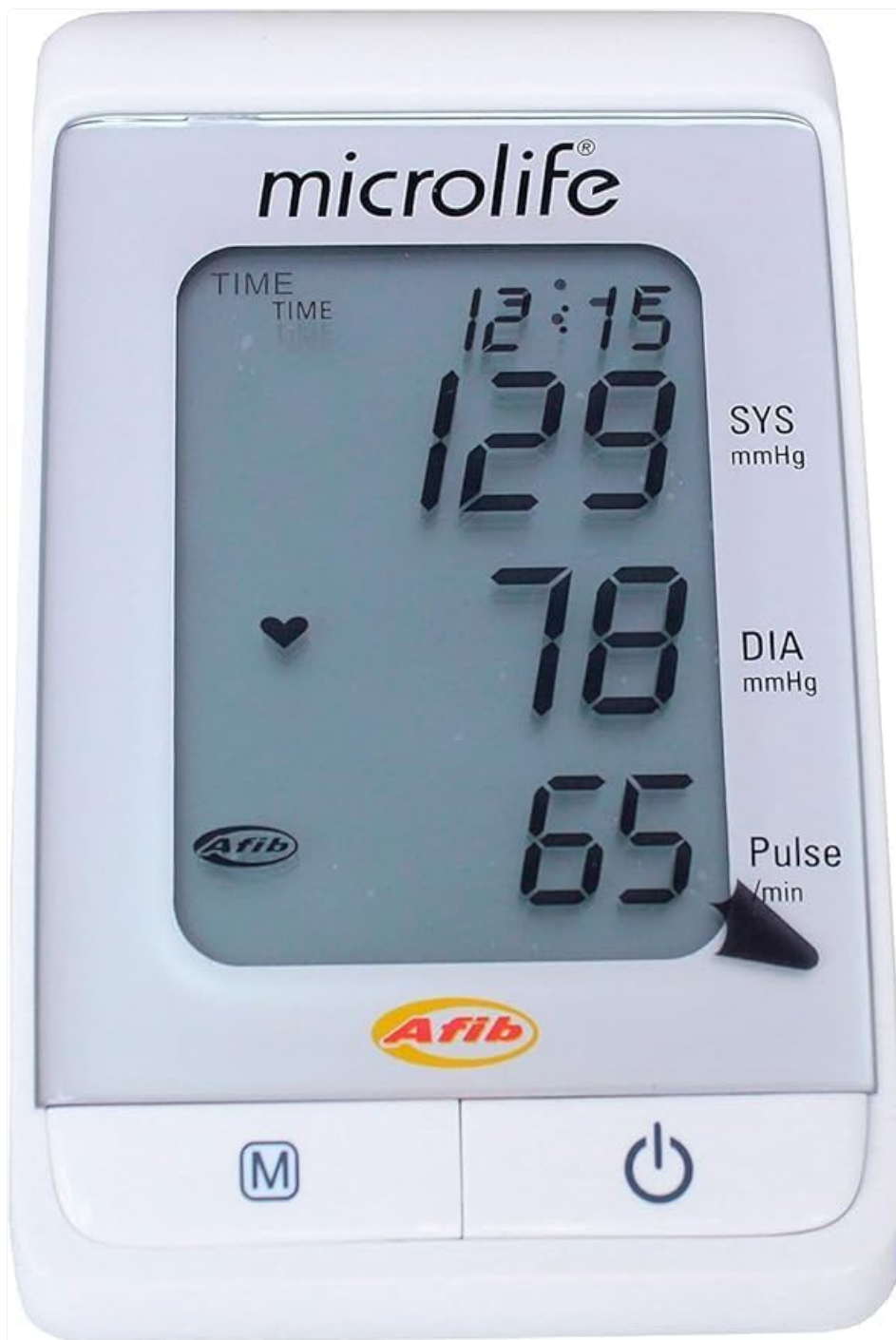
Image 3: Close-up of the monitor display showing SYS, DIA, and Pulse readings, along with the AFIB indicator.
