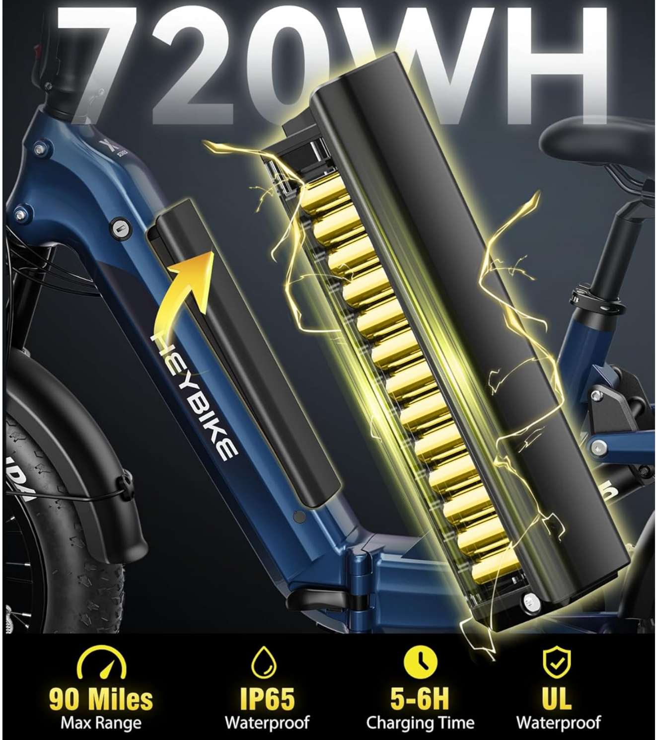
Image: Illustration of the 720WH removable battery and its integration within the bike frame.
