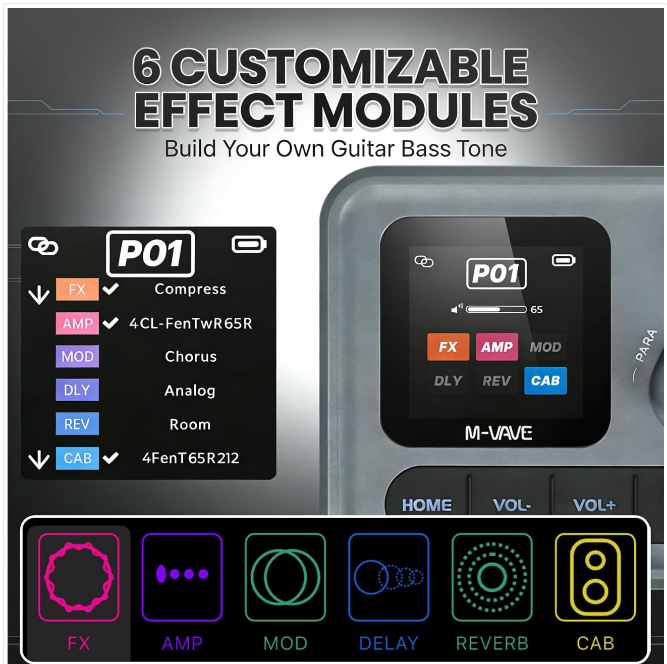
Image: A diagram illustrating the 6 customizable effect modules (FX, AMP, MOD, DLY, REV, CAB) and how they can be arranged in a signal chain on the Pocket AMP's display.
