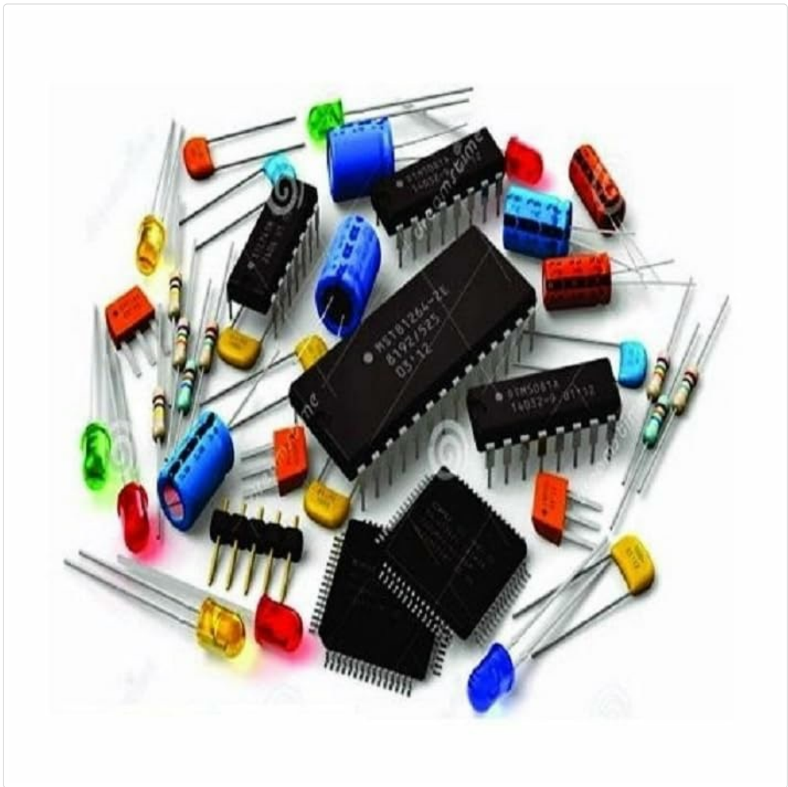
Figure 3.2: A close-up view of various electronic components typically found in the kit, including integrated circuits, capacitors, resistors, and LEDs. These are the individual parts that will be soldered onto the circuit board.
