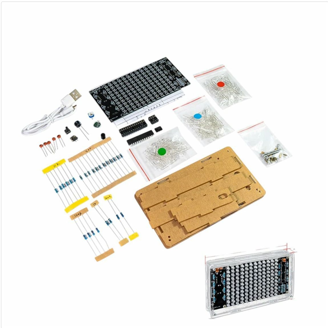
Figure 3.1: Overview of the Hu-052 LED Music Spectrum Display DIY Kit components. This image displays the main circuit board, various resistors, capacitors, LEDs, integrated circuits, a USB power cable, and acrylic casing parts, all neatly organized for assembly.
