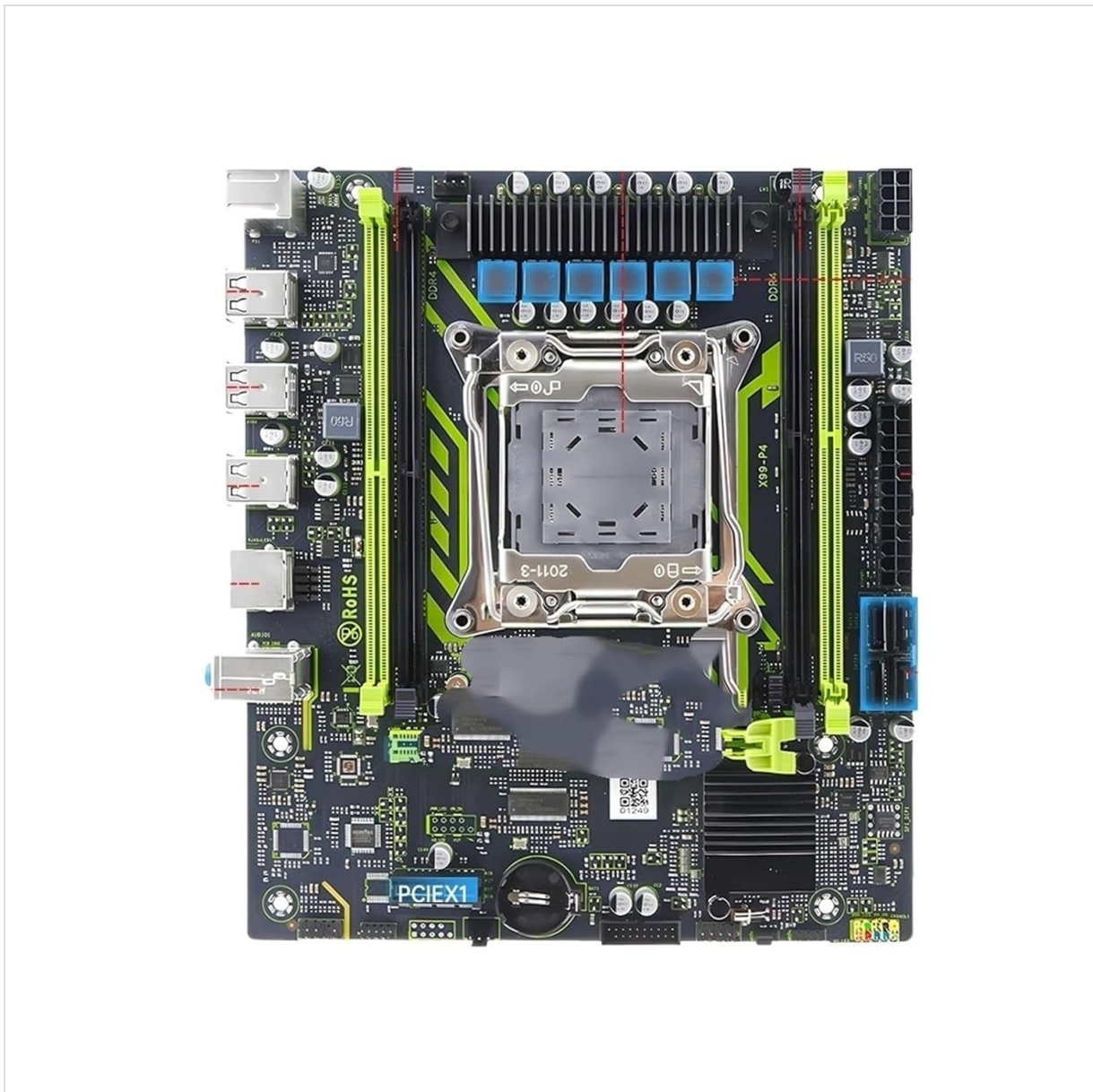
Figure 2: Detailed view of the LGA2011-3 CPU socket on the SOYO X99 Motherboard, showing the retention bracket.
