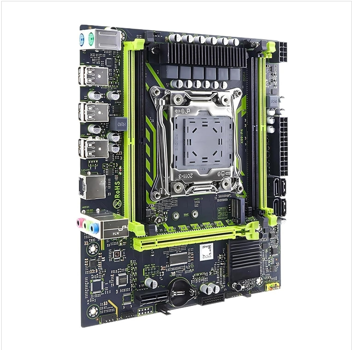
Figure 1: Top-down view of the SOYO X99 Motherboard, highlighting the LGA2011-3 CPU socket, DDR4 RAM slots, PCIe slots, and I/O ports.
