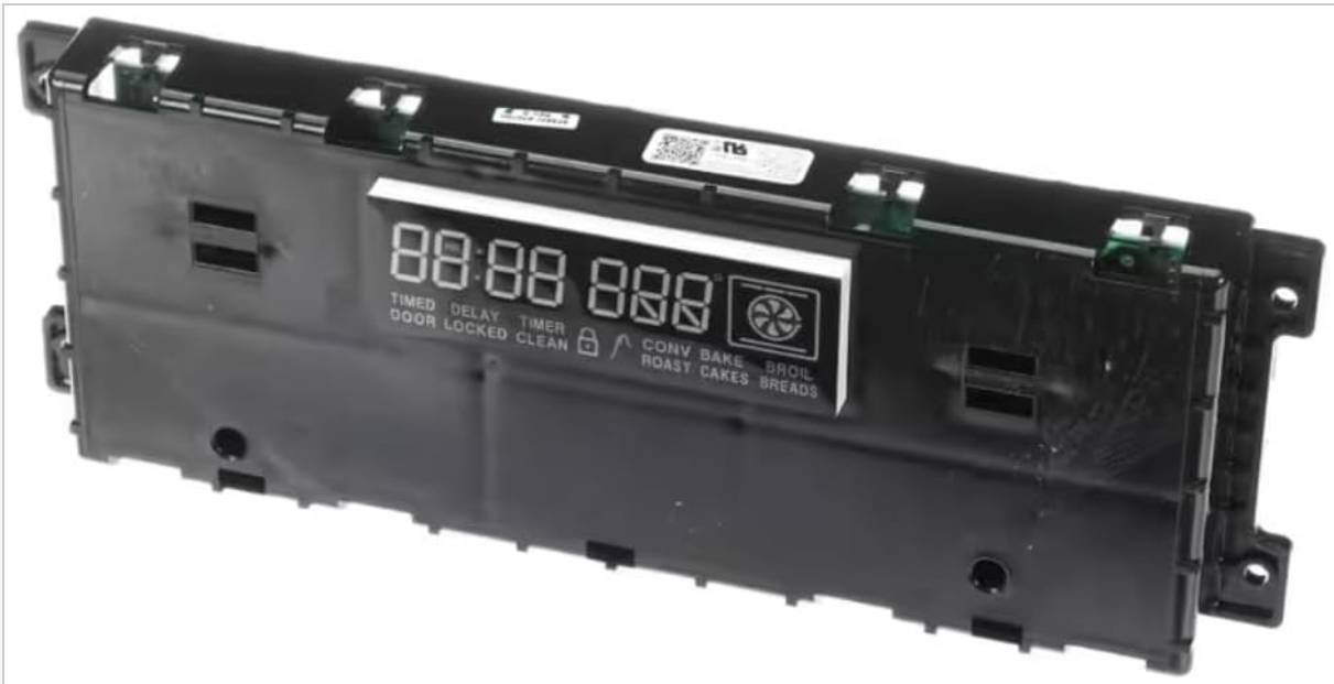
Figure 2.1: Front view of the ES585B Electronic Controller, displaying the digital clock/timer and various function indicators such as TIMED, DELAY, TIMER, DOOR LOCKED, CLEAN, CONV BAKE, BROIL, ROAST, CAKES, and BREADS.
