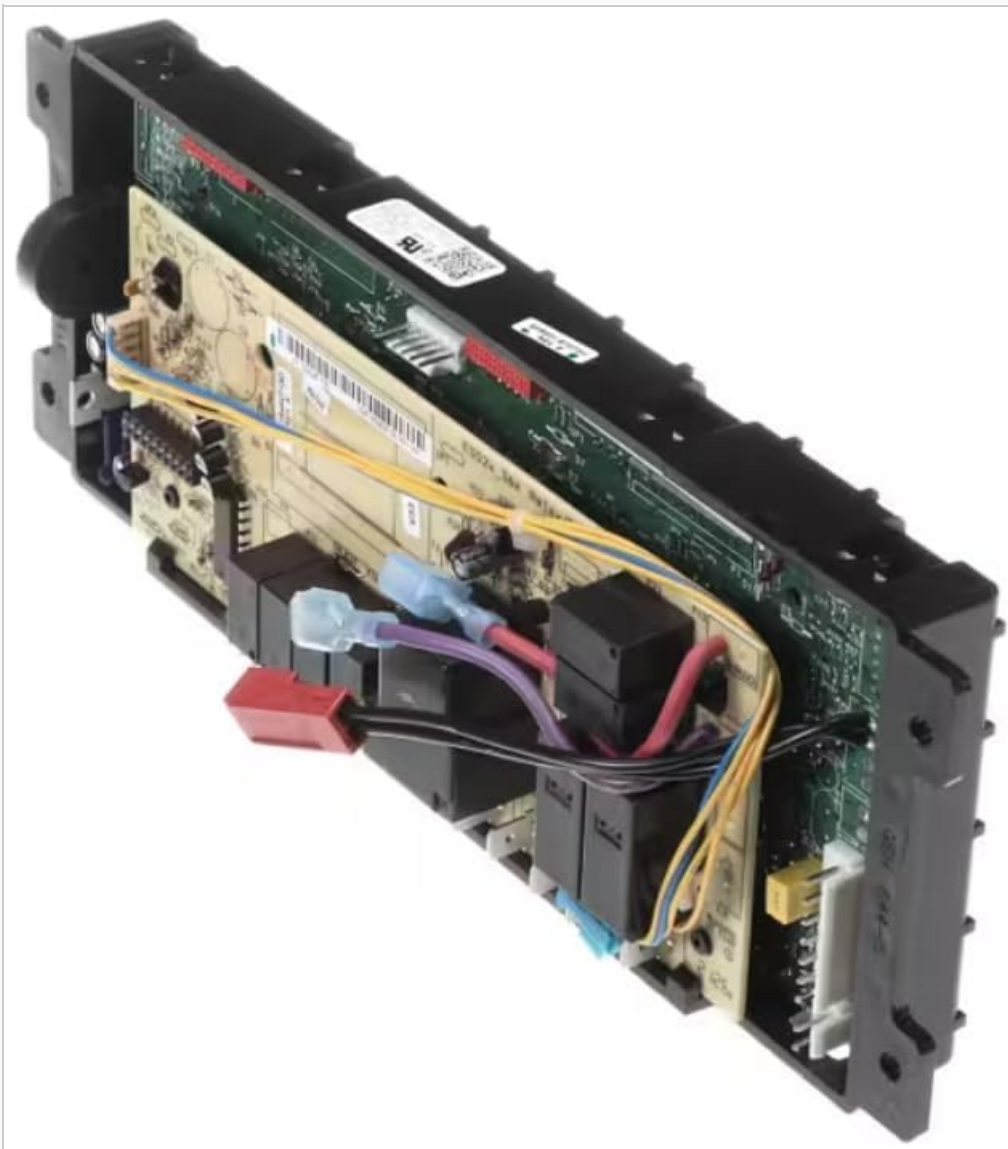
Figure 3.1: Side view of the ES585B Controller, illustrating the various wiring harnesses and connectors for integration into an appliance.
