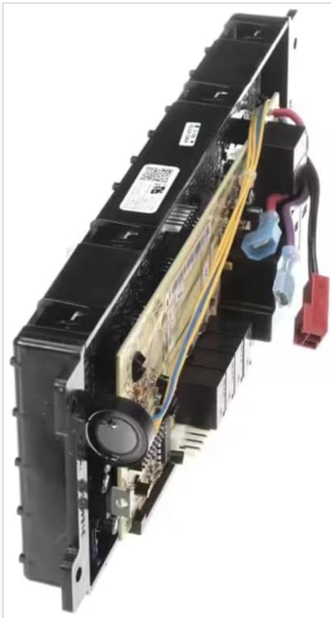
Figure 3.2: Alternate side view of the ES585B Controller, providing a different perspective on its physical structure and component placement.
