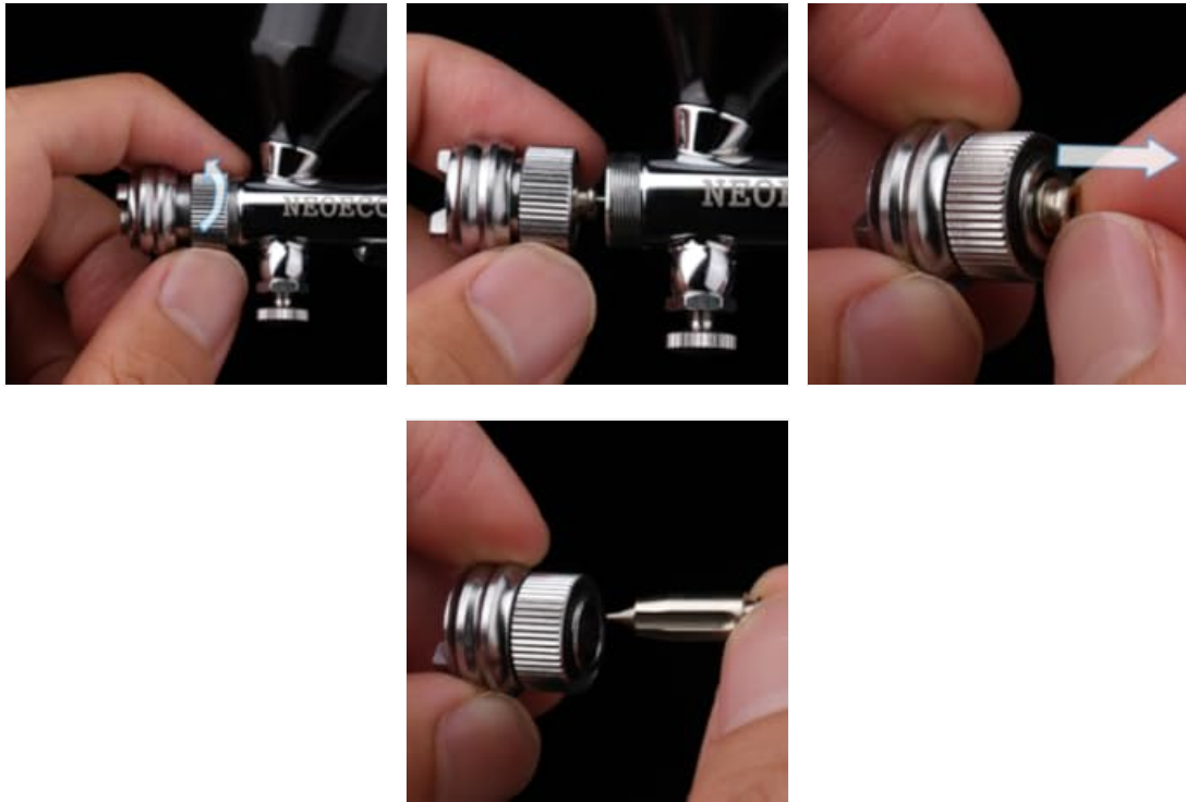
Images: Steps for removing and inserting the self-centering nozzle and needle for maintenance.
