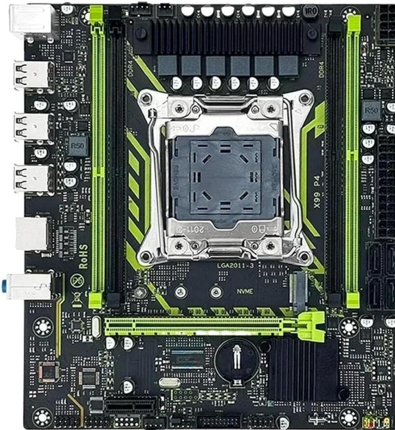
Figure 1.1: Top-down view of the SOYO X99 Motherboard, showcasing the LGA2011-3 CPU socket, DDR4 RAM slots, and various expansion ports.
