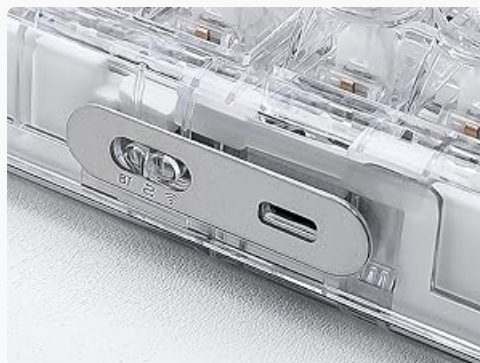
Figure 4: Close-up of the mode switch for Bluetooth (BT), 2.4G Wireless, and Wired connections.
