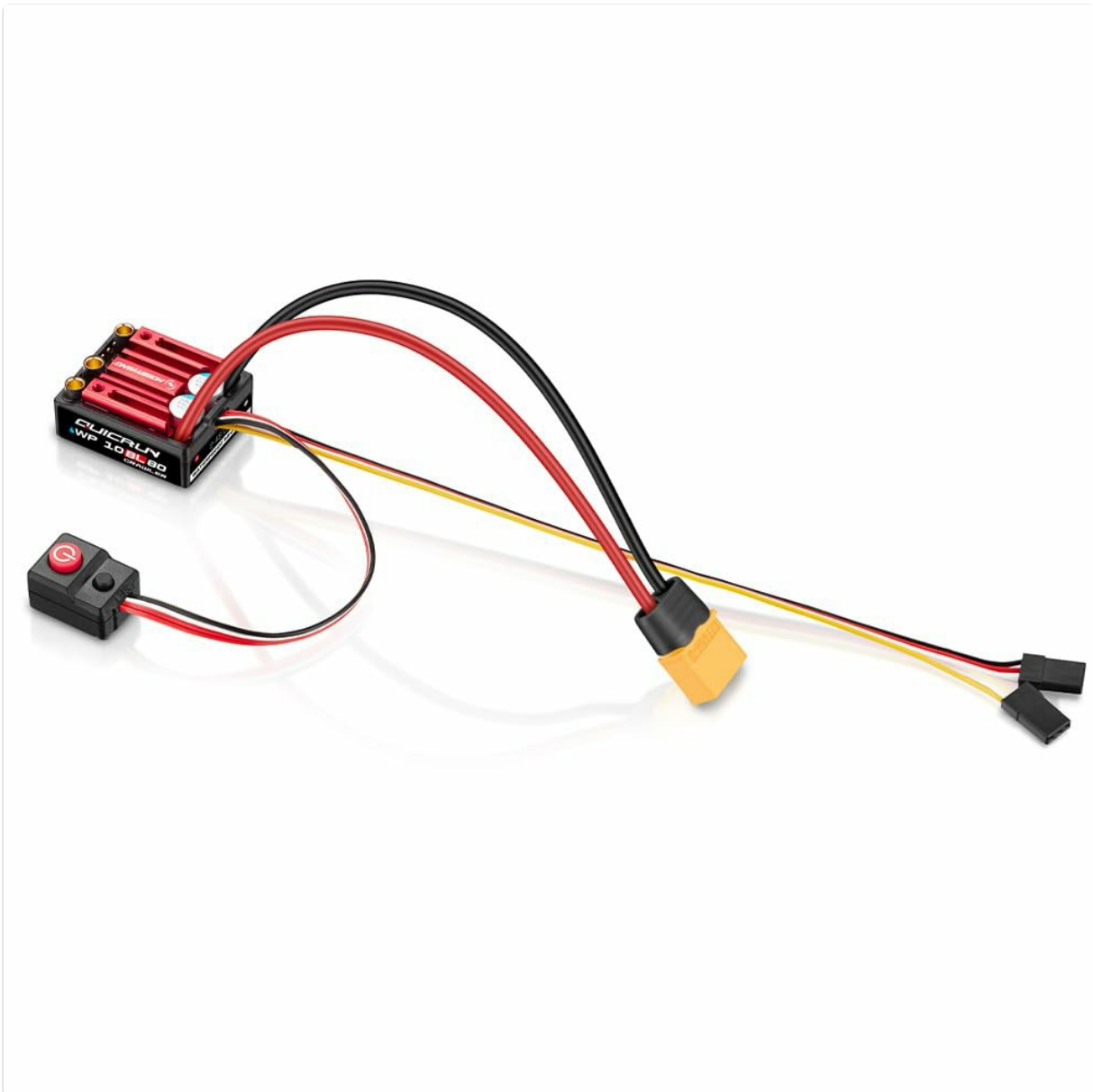
Figure 1: Hobbywing QUICRUN WP 10BL80 G2 Crawler ESC with connected wires and power switch. This image displays the main ESC unit with its red heatsink, integrated capacitors, and various wires connected, including the power input, motor output (A, B, C), and the separate power switch module with a red power button.
