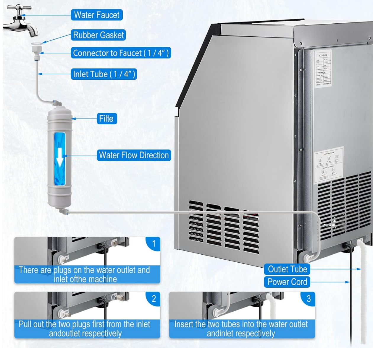
Figure 4: Water Filter and Drainage Pump Installation Diagram
