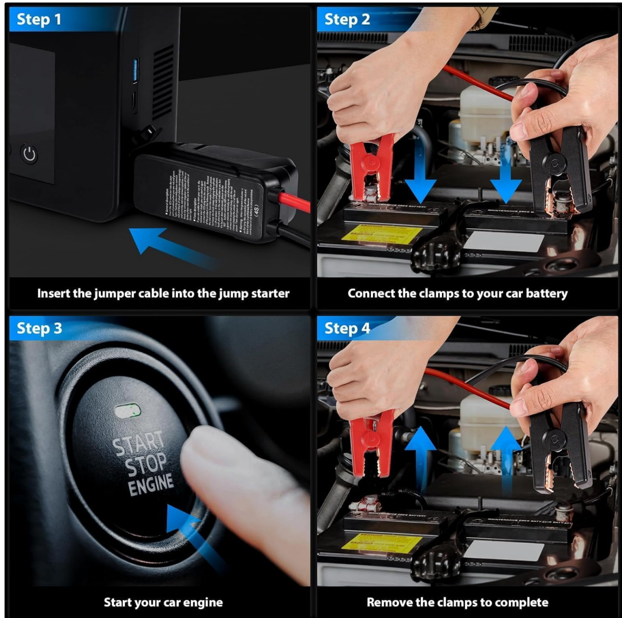
Figure 5: Illustrated steps for safely jump starting a vehicle using the Hieha L8.
