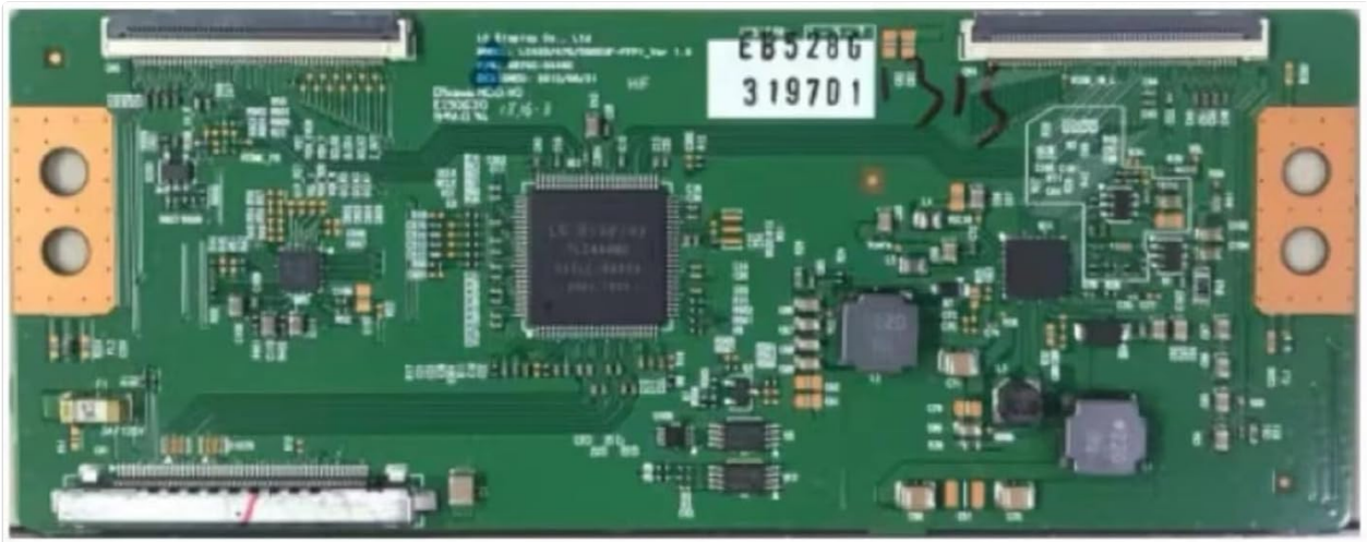
Figure 1: The GOFJAJHQ 6870C-0446C Tcon Card Logic Board. This image displays the green, rectangular circuit board populated with various electronic components including integrated circuits, capacitors, resistors, and connectors. Key identifiers such as '6870C-0446C' and 'LC420470550EUF-FFP1' are visible on the board, along with ribbon cable connectors on the top and bottom edges for connecting to the display panel and main board.
