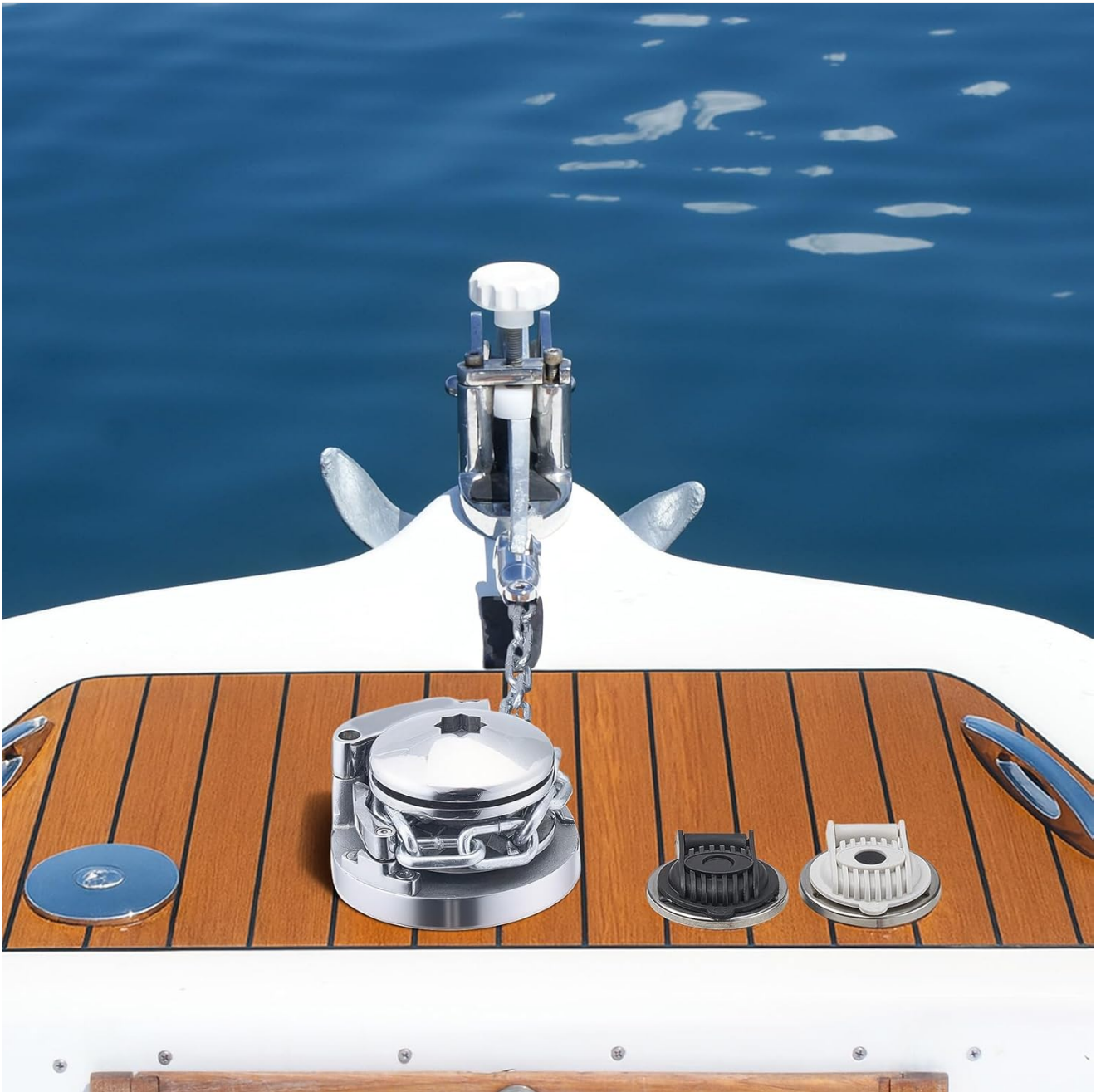
Image 5.2: Properly installed windlass with anchor chain.
