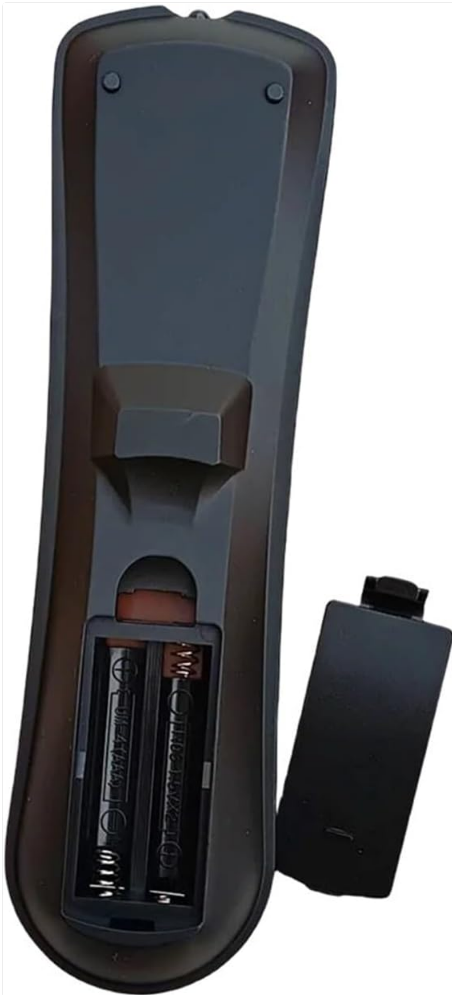
Figure 2: Close-up view of the remote control's battery compartment, showing the correct orientation for AAA battery insertion.
