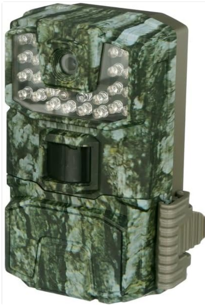
Figure 4.2: Front view of the Bushnell Spot On Trail Camera. This image displays the camera lens, the motion sensor, and the array of Low Glow IR LEDs for night vision.
