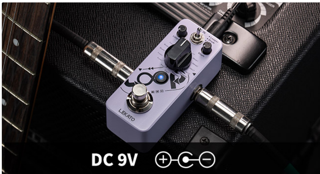
Figure 6: Power connection for the pedal (DC 9V center negative).
