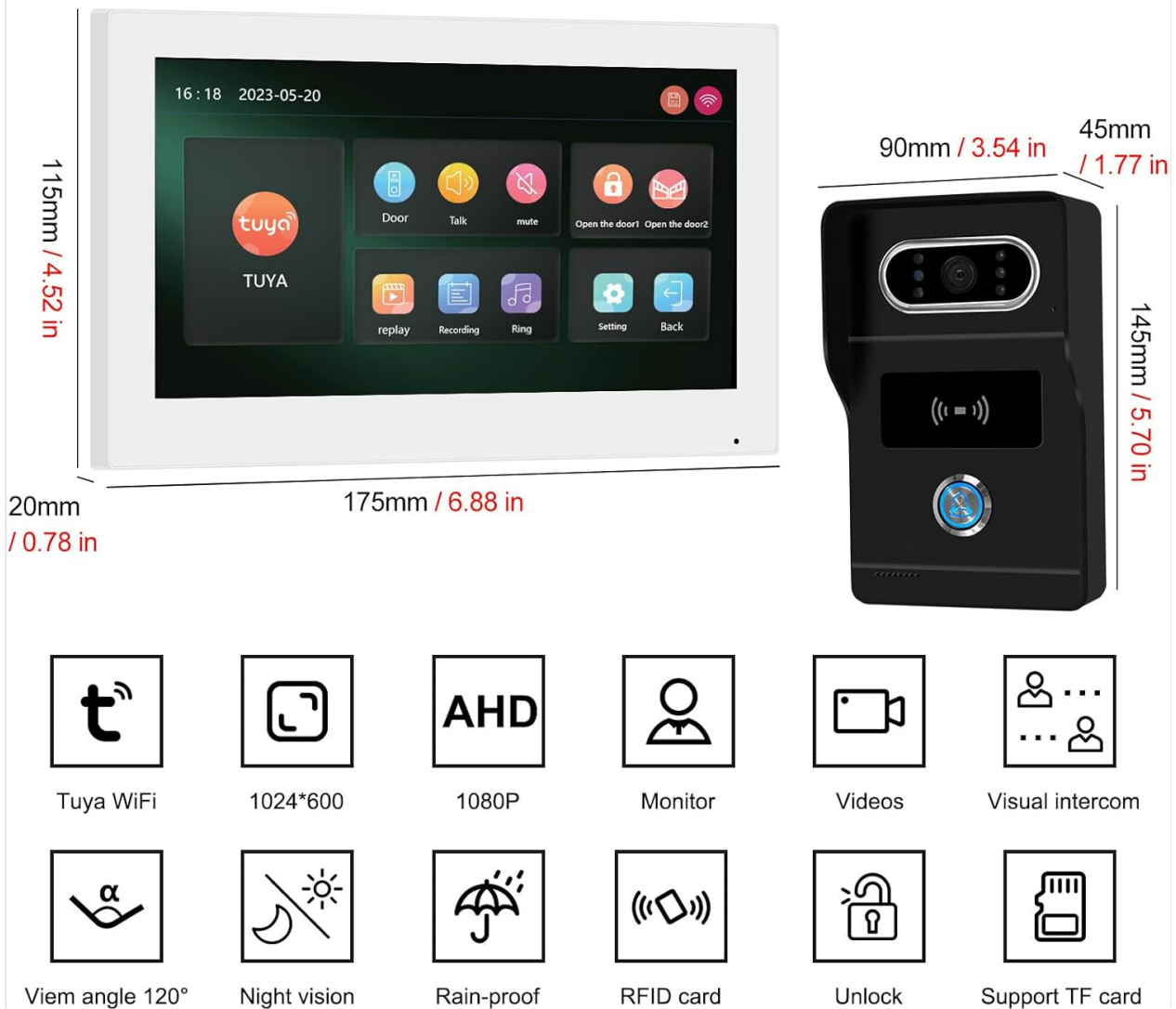
Figure 4.1: Dimensions and Key Features Overview. This image illustrates the physical dimensions of both the indoor monitor (175mm x 115mm x 20mm) and the outdoor unit (90mm x 145mm x 45mm), alongside a visual summary of features including Tuya Wi-Fi, 1024*600 resolution, AHD, 1080P camera, 120° viewing angle, night vision, rain-proof design, RFID card support, unlock function, and TF card support.
