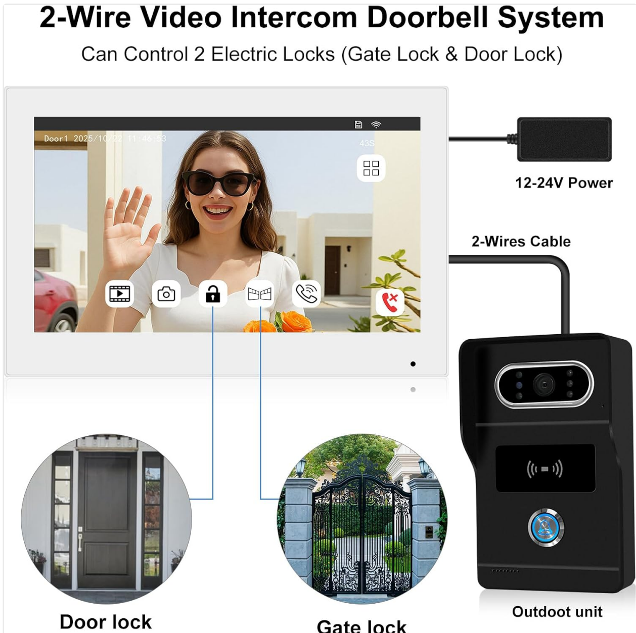
Figure 5.1: 2-Wire Video Intercom Doorbell System Wiring. This diagram illustrates how the indoor monitor connects to a 12-24V power source and the outdoor unit via a 2-wire cable. It also shows the connections for controlling two electric locks: a door lock and a gate lock.
