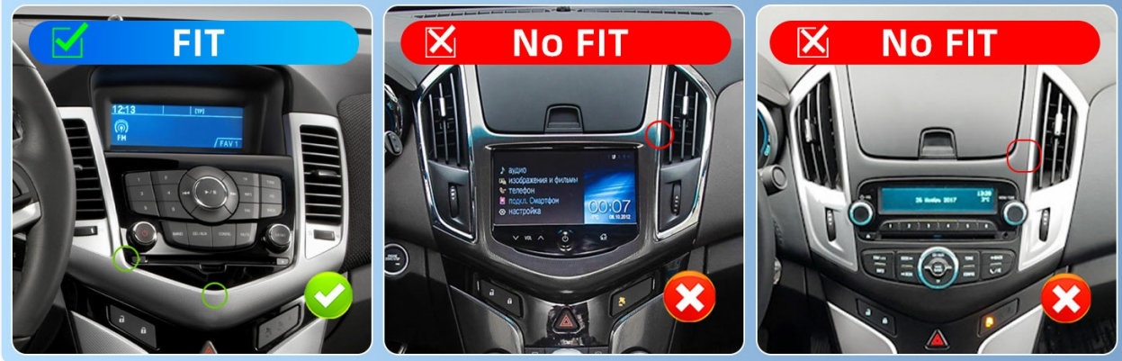
Image 3.1: Visual guide for checking dashboard compatibility. The 'FIT' example shows the correct original car system configuration for installation, while 'No FIT' examples illustrate incompatible layouts.
