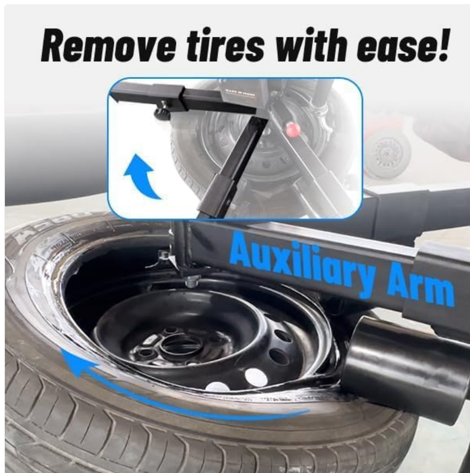
Figure 5.2: Auxiliary Arm in Use. The auxiliary arm is shown here facilitating the removal of a tire from the rim, demonstrating its role in simplifying the process.
