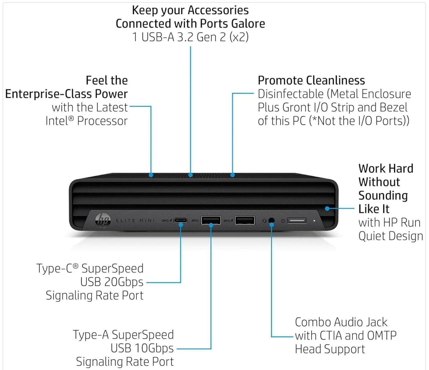
Figure 2: Front Panel Ports and Features
