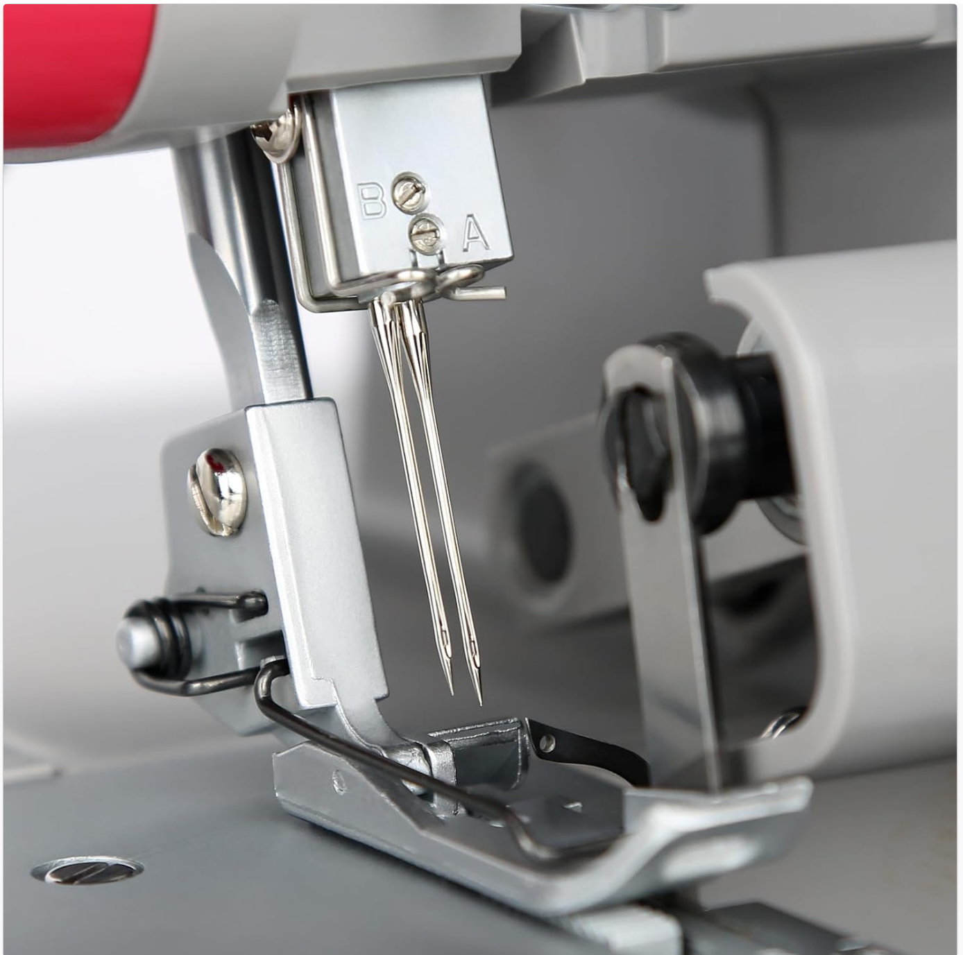
Figure 2.2: Close-up view of the serger needles. This image shows the needle area, indicating where needles are inserted and their typical arrangement.
