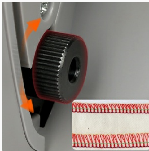
Figure 3.4: Cutting Width Adjustment. This image shows the lever used to adjust the cutting width, allowing for precise trimming of fabric edges.
