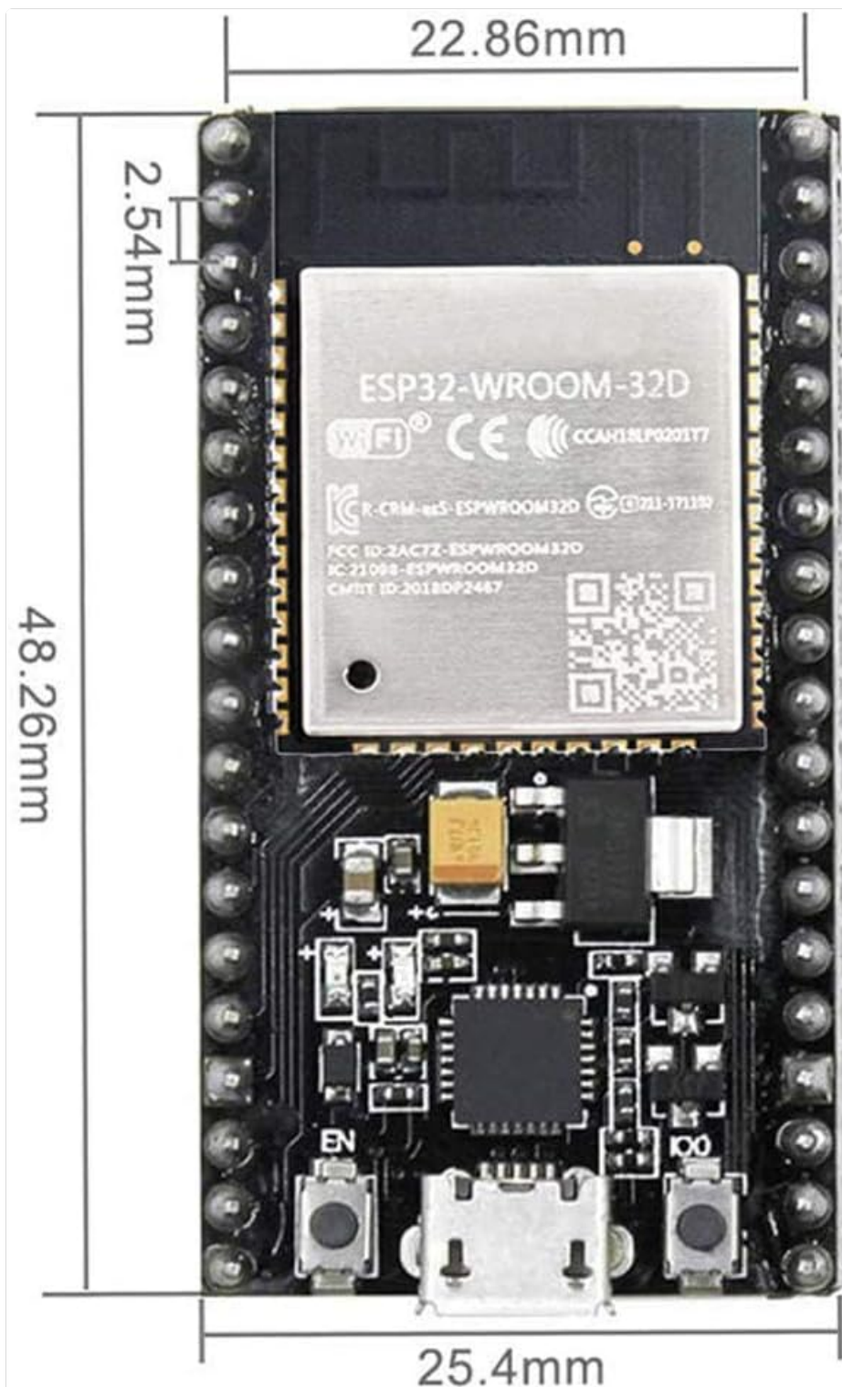
Figure 7.1.2: Detailed top view of the ESP32-S Development Board with dimensions.
