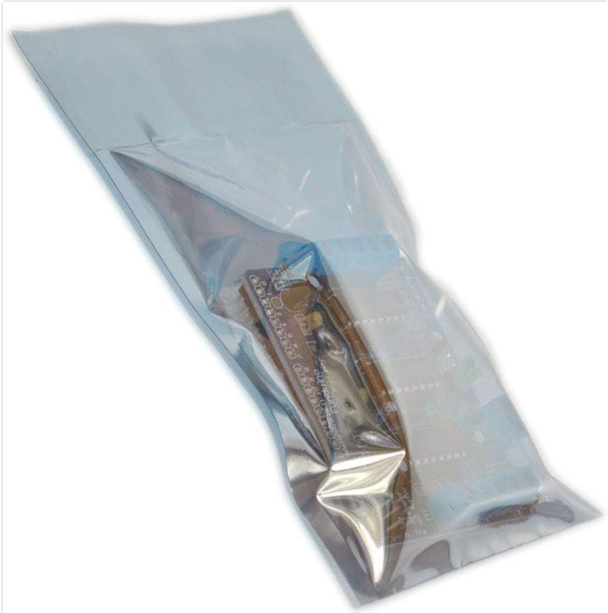
Figure 3.1: The HiLetgo L293D Motor Drive Shield typically comes in an anti-static bag for protection.
