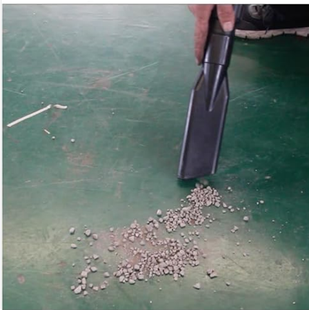
Figure 5.3: Wet Vacuuming in Progress. This image demonstrates the vacuum effectively cleaning a wet floor with various debris, showcasing its wet pickup capability with the front-mounted squeegee.
