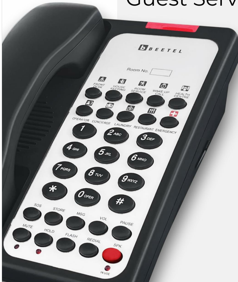
Figure 4: 10 Programmable Guest Service Keys. This image displays the dedicated keys for various guest services on the phone's keypad.
