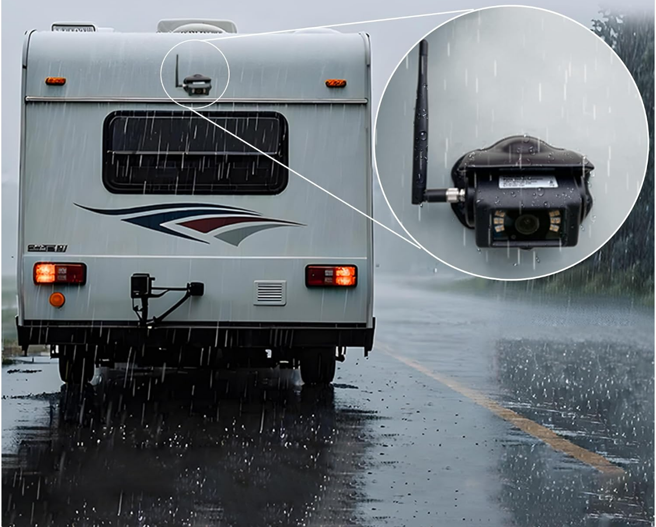
Figure 3.2: Wireless rear camera installation on an RV.
