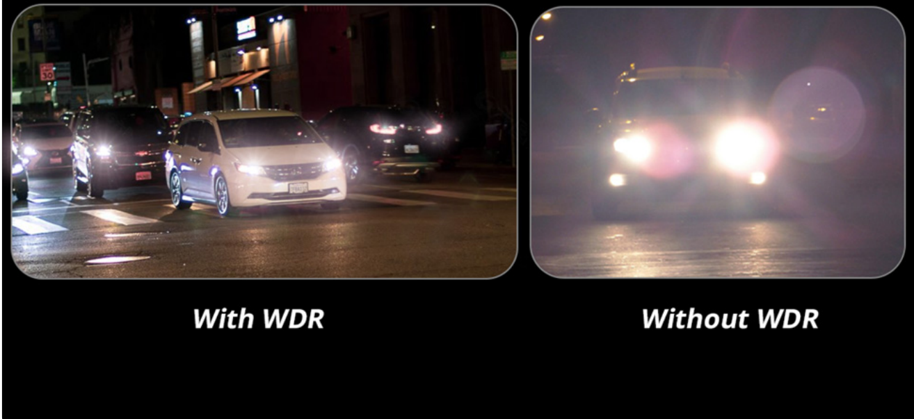
Figure 4.2: Wide Dynamic Range (WDR) technology comparison.
