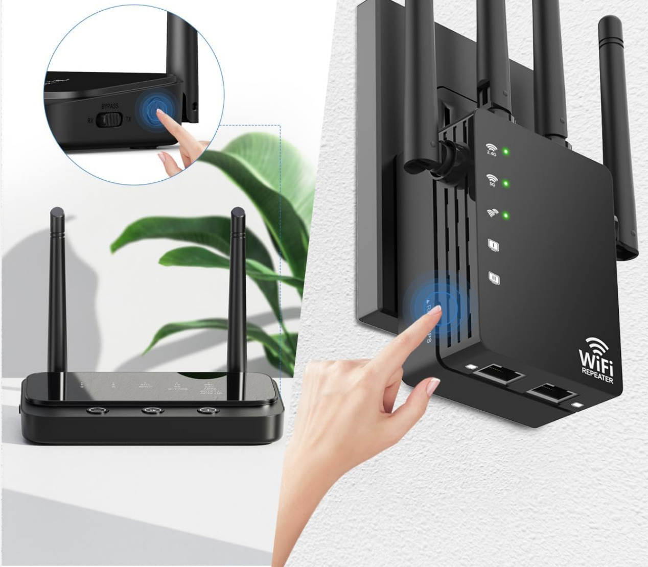
Figure 3: WPS Setup. This image demonstrates the simple WPS setup process, showing a hand pressing the WPS button on both a router and the GEYILO WiFi Extender.
