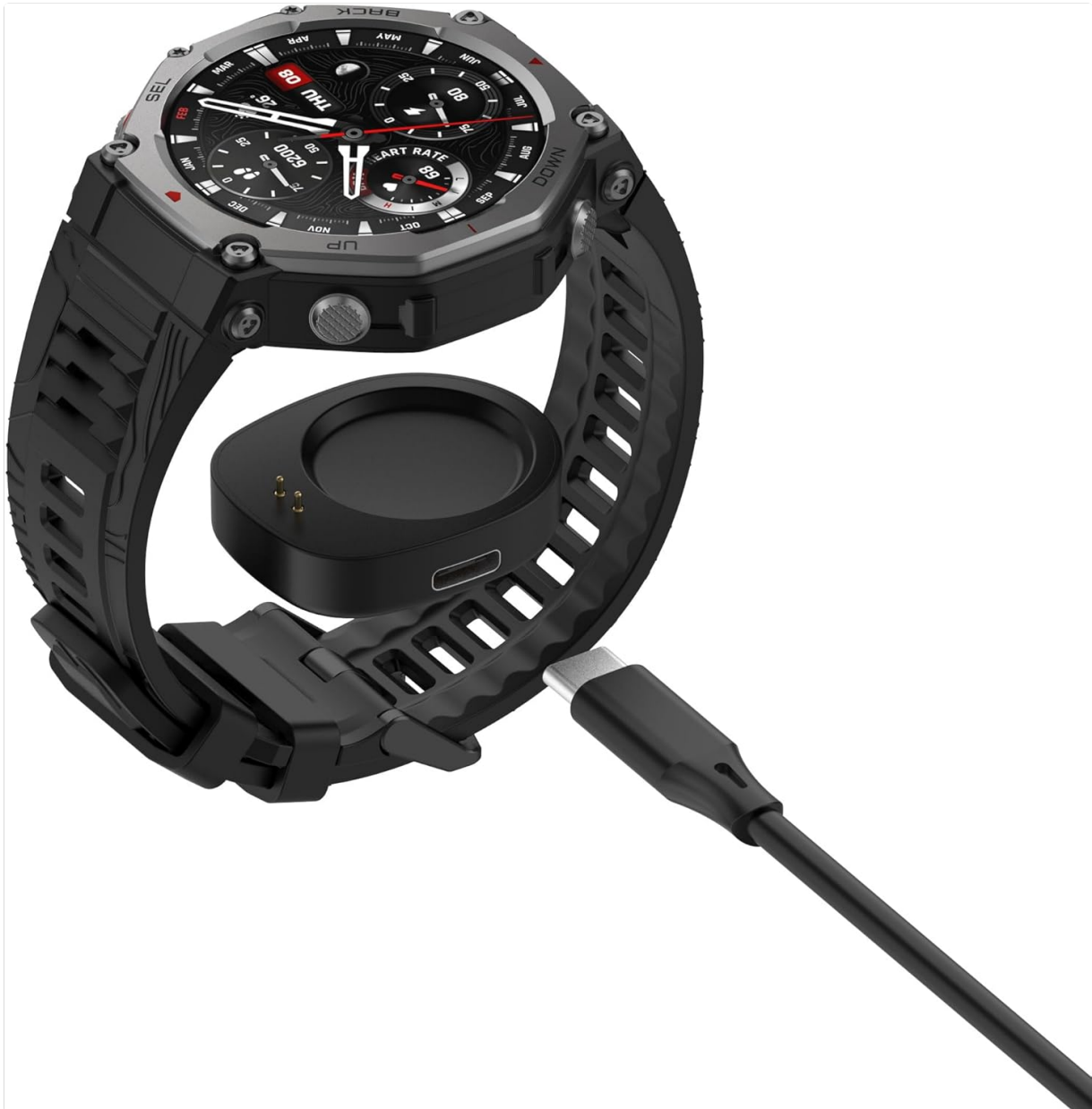
Image 3.1: An Amazfit smartwatch positioned next to the charging dock, with the Type-C cable being connected to the dock's input port.
