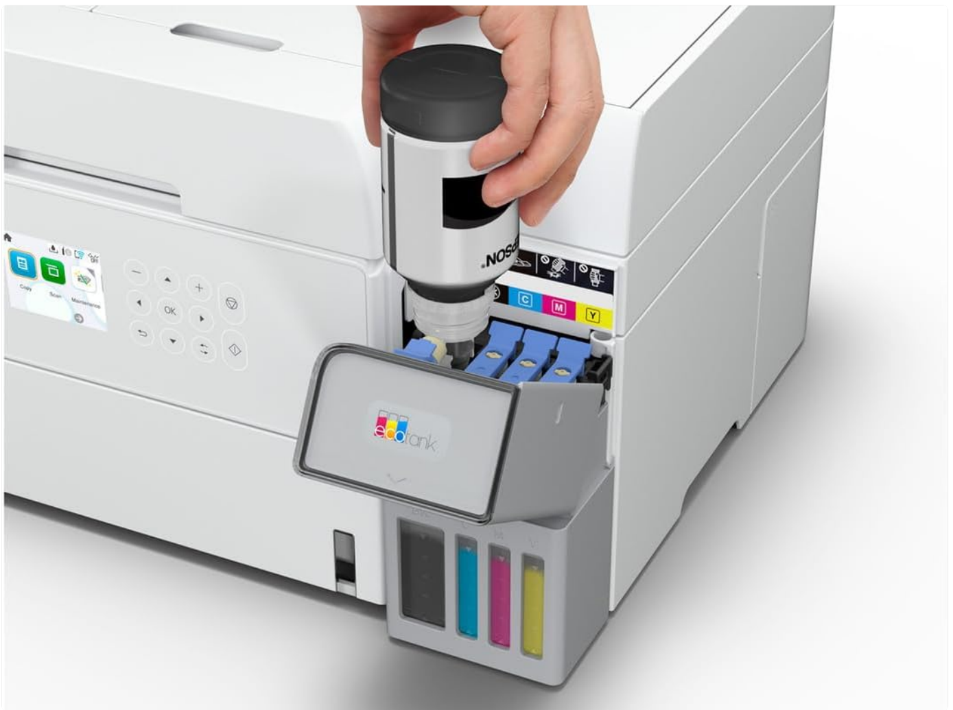
Figure 2.3.1: Filling the black ink tank. Ensure the correct color ink bottle is used for each tank.
