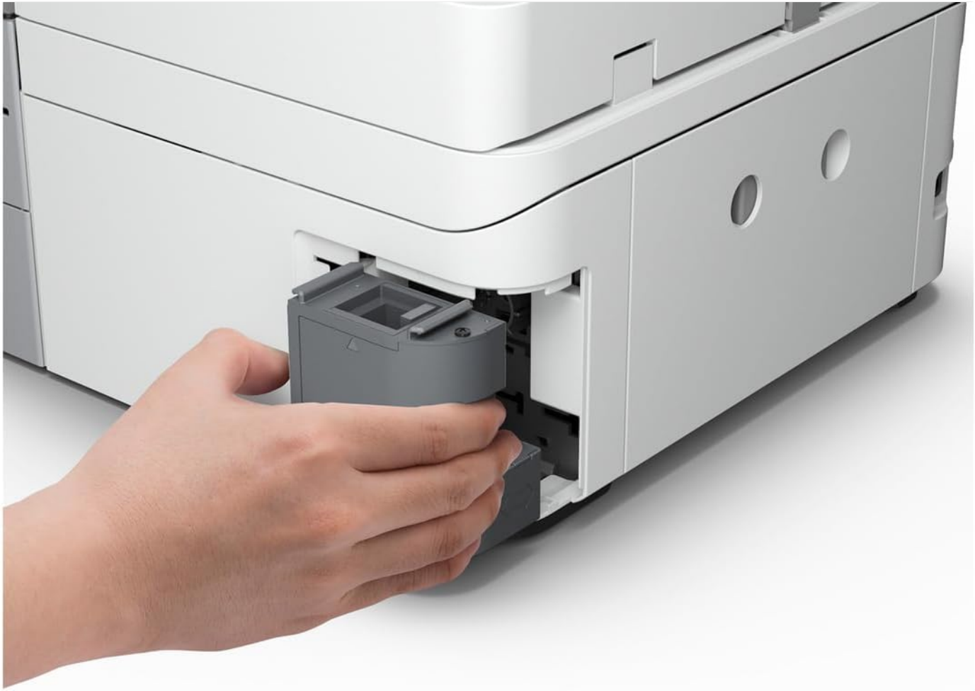
Figure 4.3.1: Removing the maintenance box for replacement.
