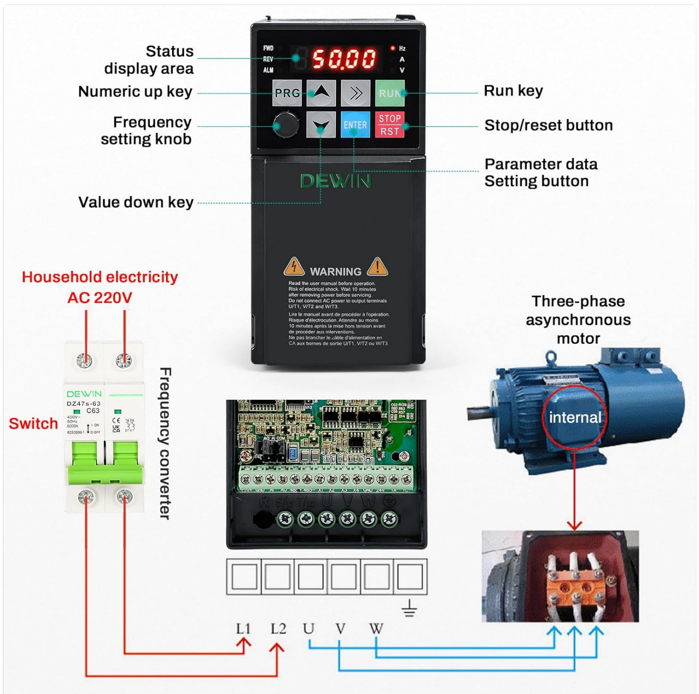
Figure 5.5: Overview showing the VFD control panel, connection to household AC 220V electricity via a switch, and wiring to a three-phase asynchronous motor.
