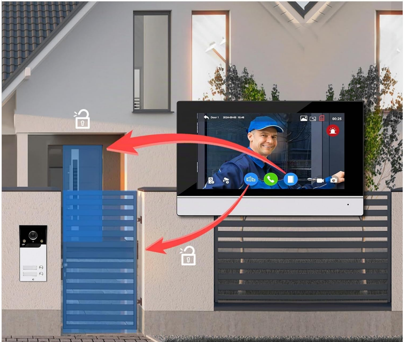
Figure 3.1.2: Controlling Two Locks. This image illustrates the monitor's capability to control two distinct electric locks, such as a gate lock and a door lock, with a single touch.
