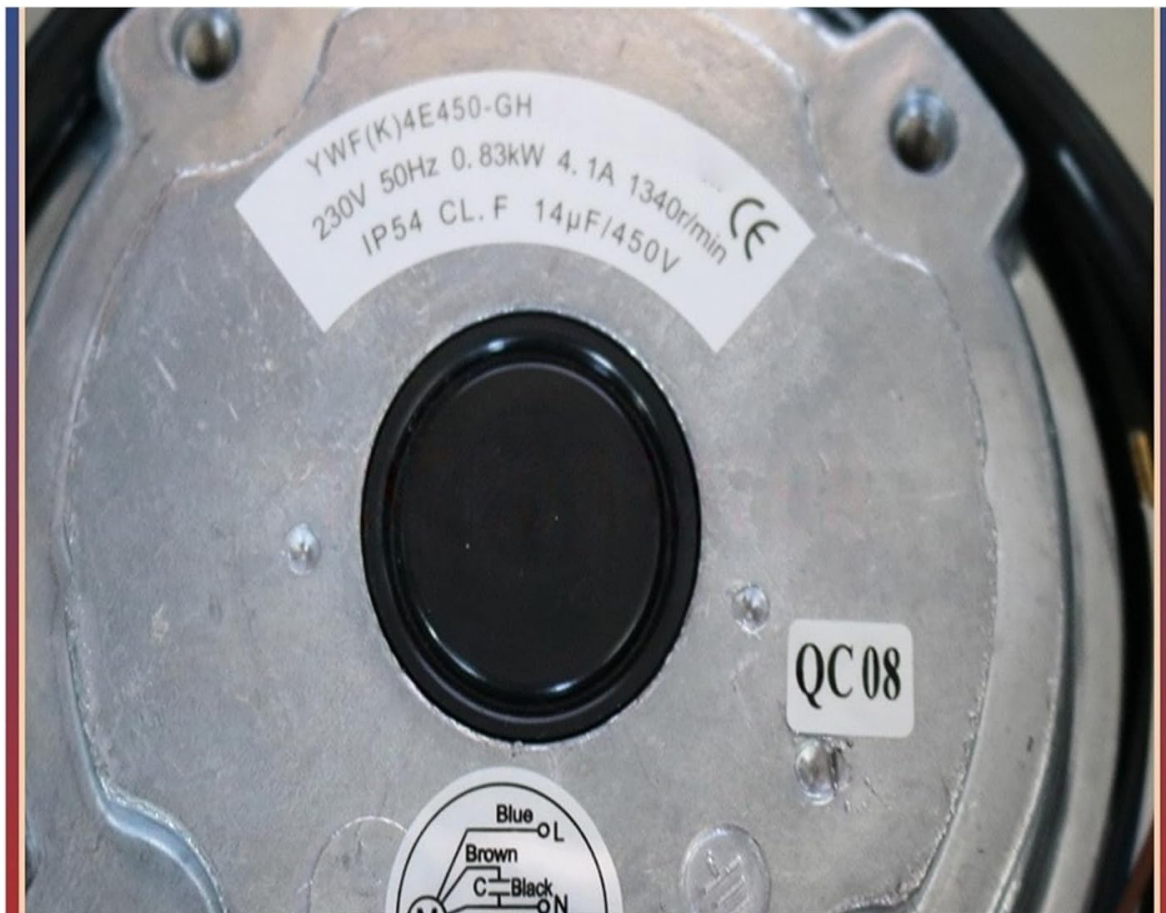
Figure 4.3: Close-up of the motor label, displaying critical electrical specifications (230V 50Hz, 0.83KW, 4.1A, 1340r/min, IP54, CL. F, 14uF/450V) and wiring color codes (Blue, Brown, Black) for proper electrical connection.
