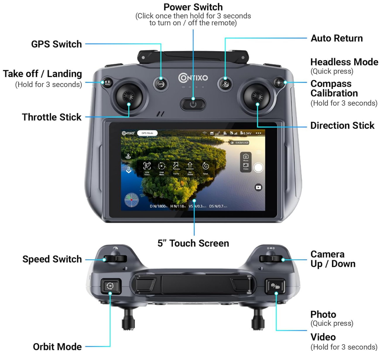
Image: Detailed layout of the Contixo F29 Drone's remote control, with labels for each button and joystick function.
