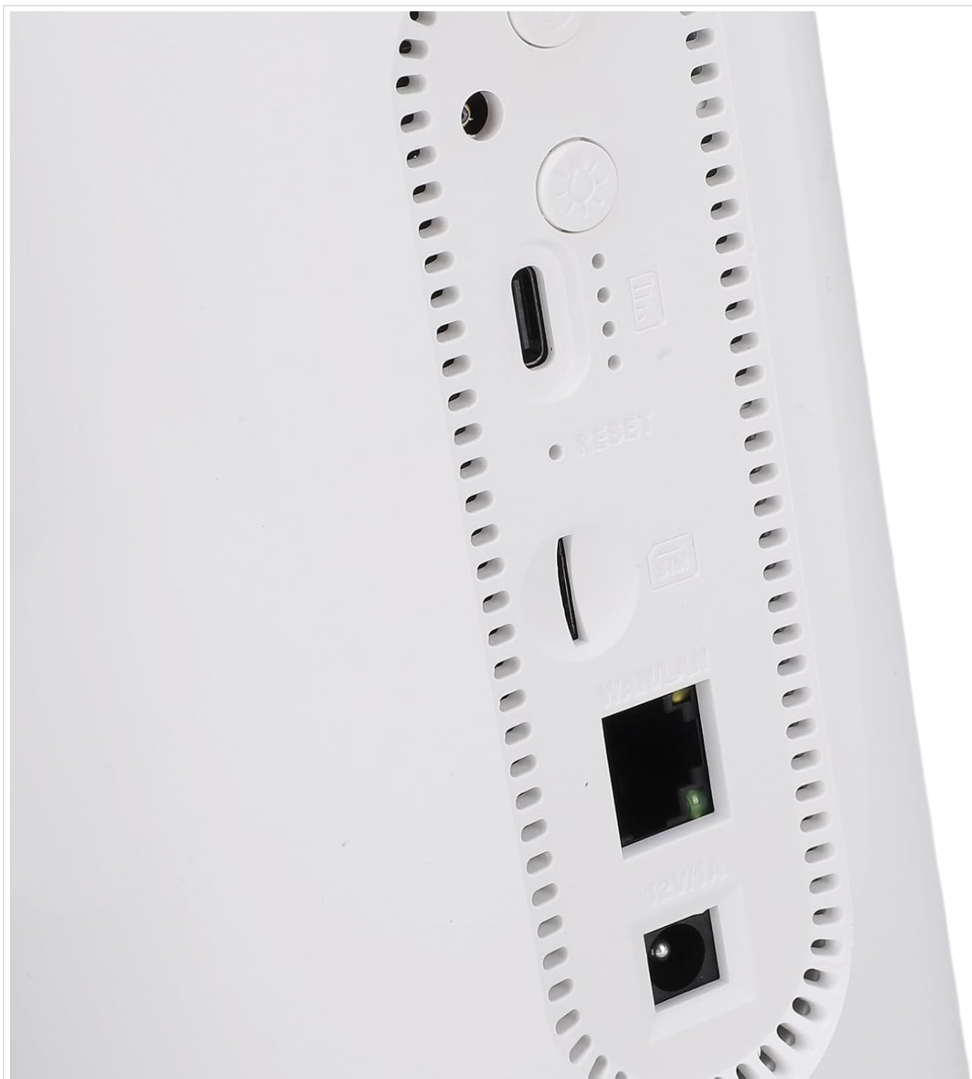
Image: Close-up view of the rear ports, including SIM card slot, Reset button, WAN/LAN port, and power input.
