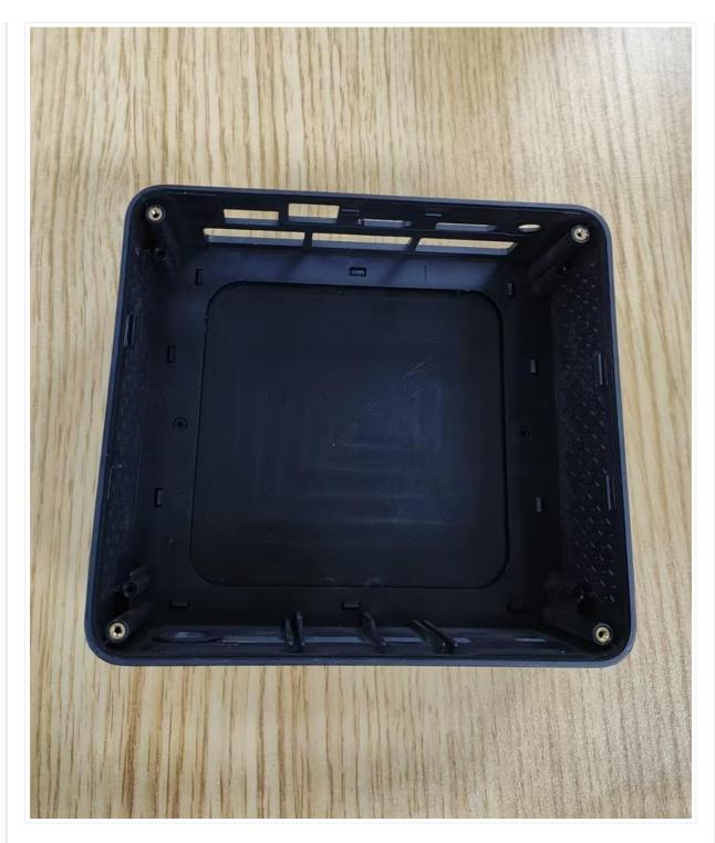
This image displays the internal housing of the Bmax Mini PC B1 Pro, showing the structural components and mounting points within the device's casing. It illustrates the design of the enclosure without the internal electronic components installed.
