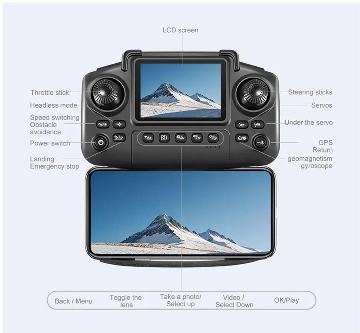
Image 4.3: Detailed diagram of the remote control functions.
