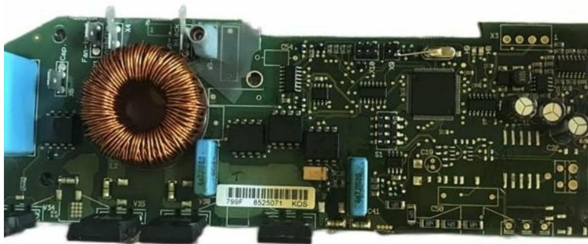
Figure 1: Overview of the PC00299 G 799F electronic component. Key features include a prominent copper inductor coil, multiple capacitors (e.g., blue cylindrical ones), and various integrated circuits. Connectors such as X3, X4, X5 are visible, along with labels like "Cap", "Fan-t", "V35", "V38", "799F", "8525071", and "KOS".
