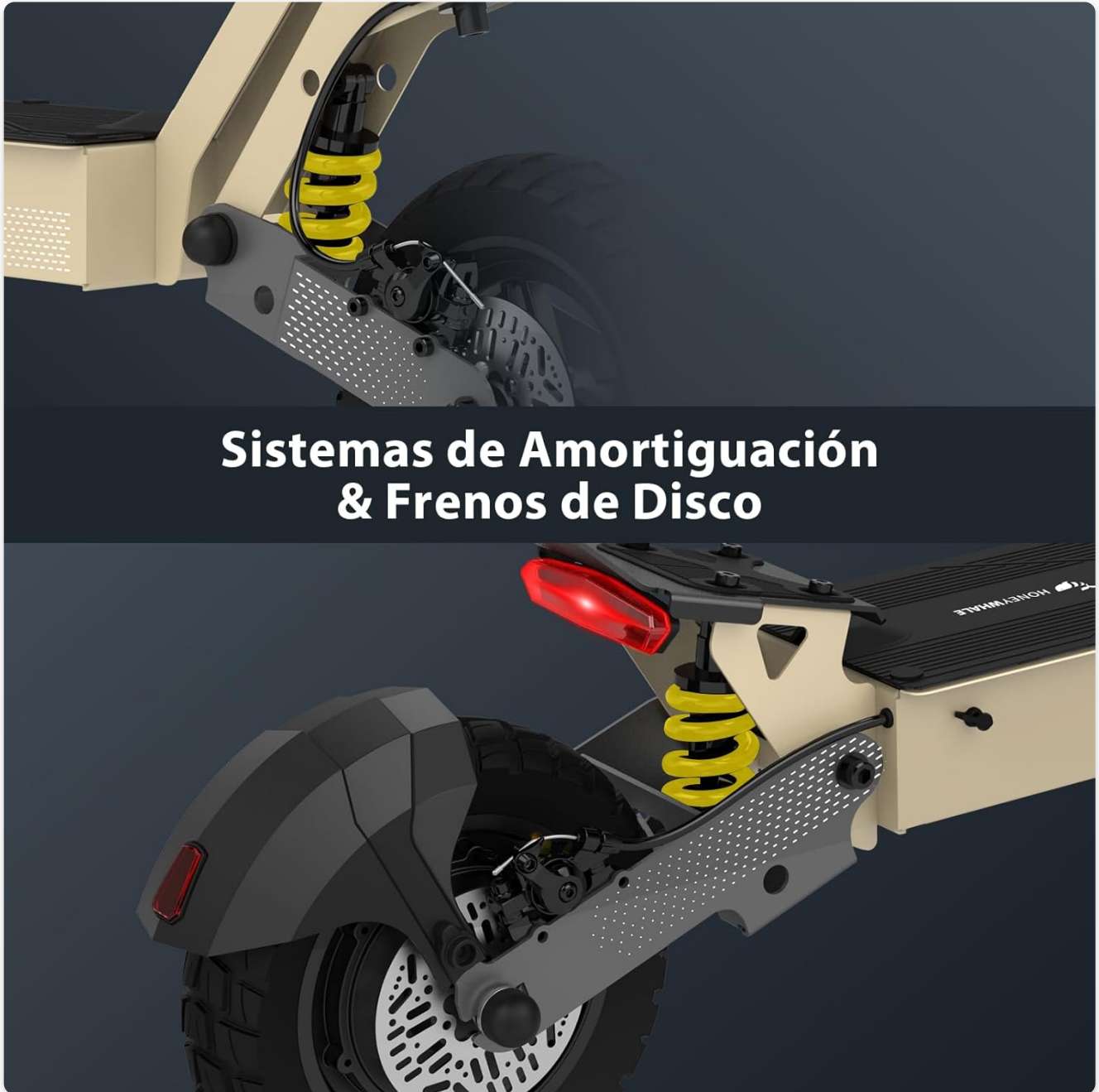
Figure 5: Suspension and Disc Brake Systems. This image displays the scooter's dual suspension system and disc brakes, emphasizing comfort and safety. The top part shows the front suspension, and the bottom part shows the rear suspension and disc brake.
