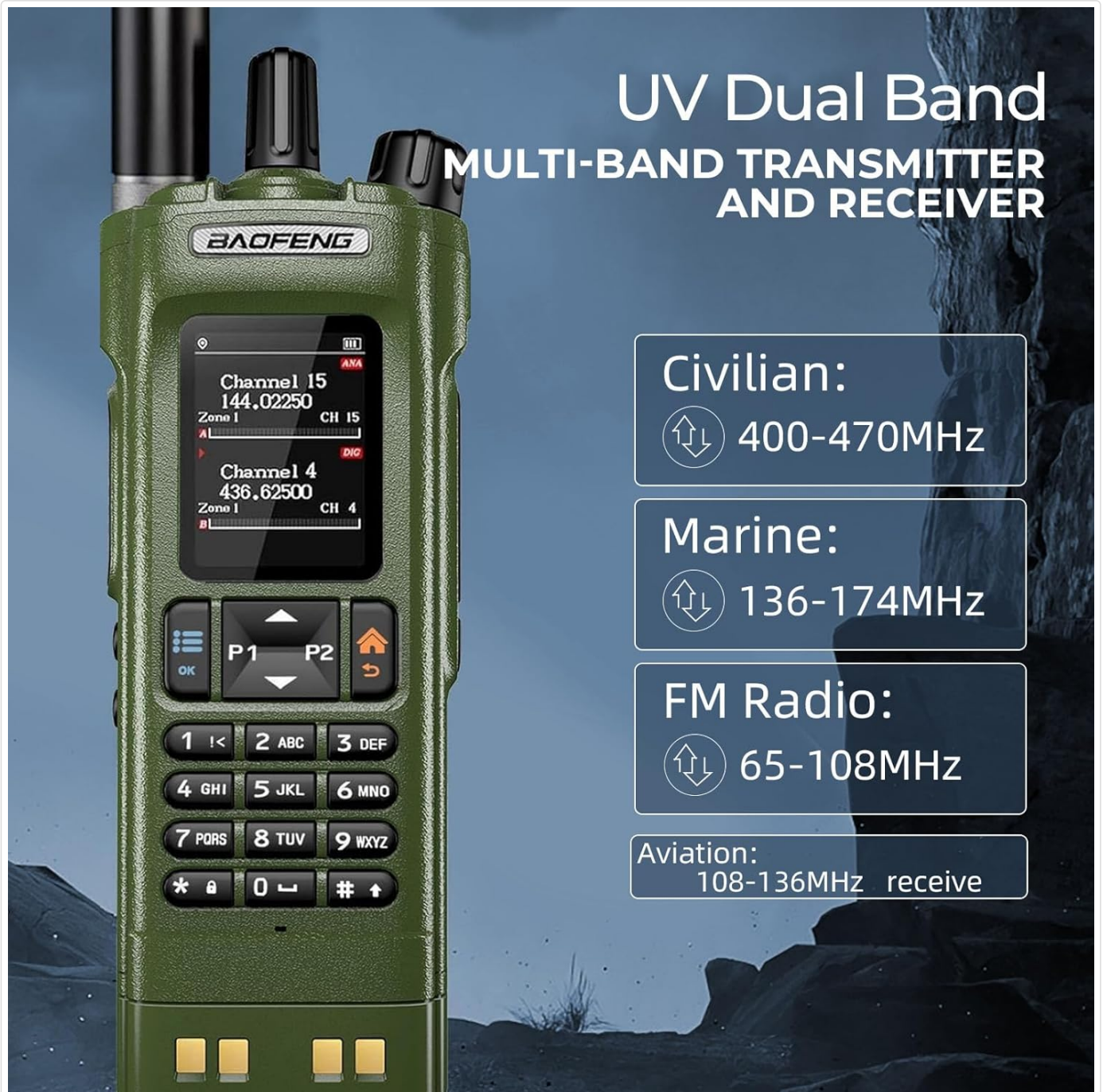
Image: The BAOFENG DM32 DM-32UV radio highlighting its UV Dual Band capabilities, specifying frequency ranges for Civilian, Marine, FM Radio, and Aviation (receive) use.
