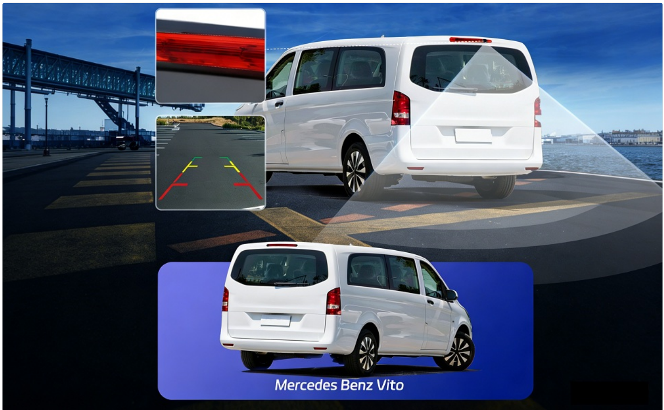
Image 1.2: Integrated brake light camera with a 140-degree wide-angle lens for comprehensive rear visibility.
