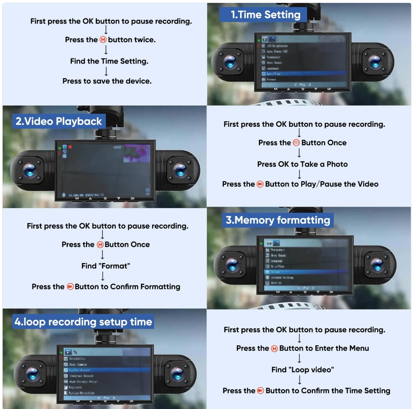
Figure 8: Overview of key menu settings for time, video playback, memory management, and loop recording.
