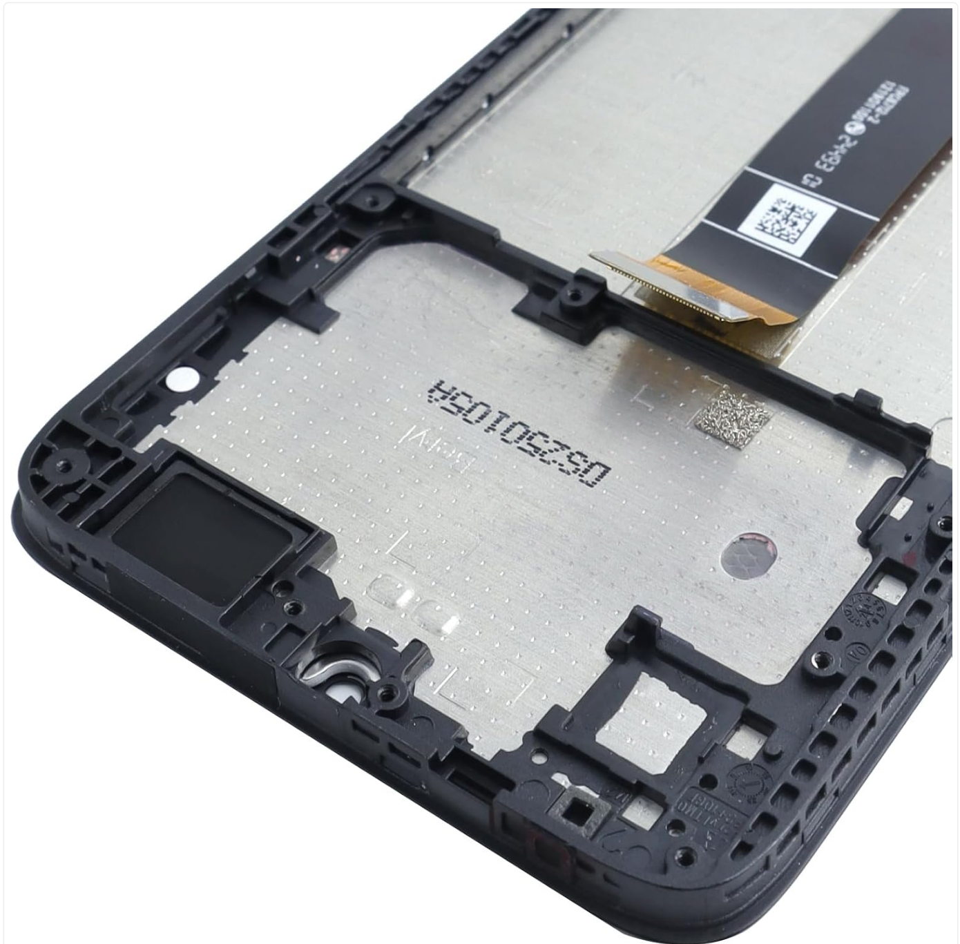
Image: Detailed view of the upper section of the display assembly, highlighting the frame structure and flex cable connection points.
