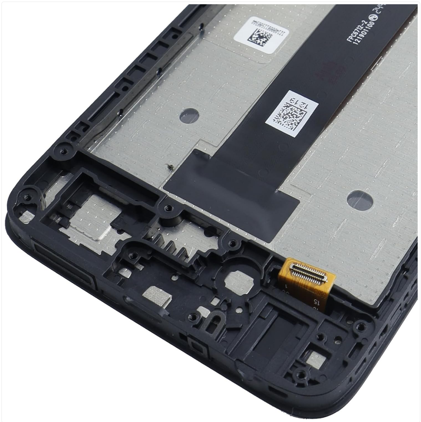
Image: Detailed view of the lower section of the display assembly, showing the frame structure and flex cable connection points.
