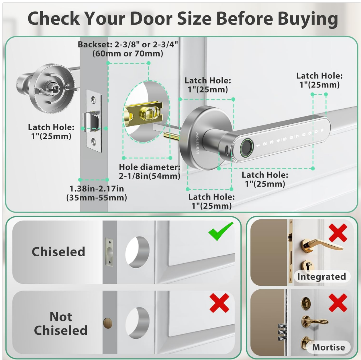
Image 4.1: This image provides critical measurements for door compatibility, showing the required backset (2-3/8 or 2-3/4 inches), latch hole diameter (1 inch), and door hole diameter (1.38-2.17 inches). It also indicates suitable door types (chiseled) and unsuitable types (integrated, mortise).
