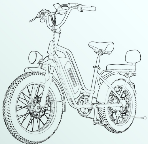
Image 5.7: Diagram highlighting the 180mm mechanical disc brake system, designed for faster braking and shorter stopping distances.
