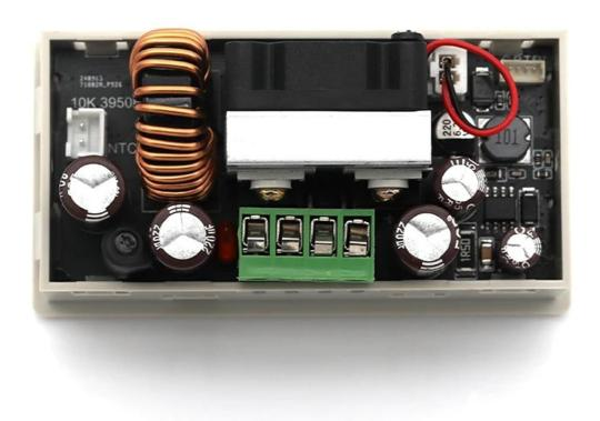
**Figure 3:** Internal view of the module showing the input/output screw terminals, inductor, capacitors, and cooling fan. Ensure secure connections to these terminals.
