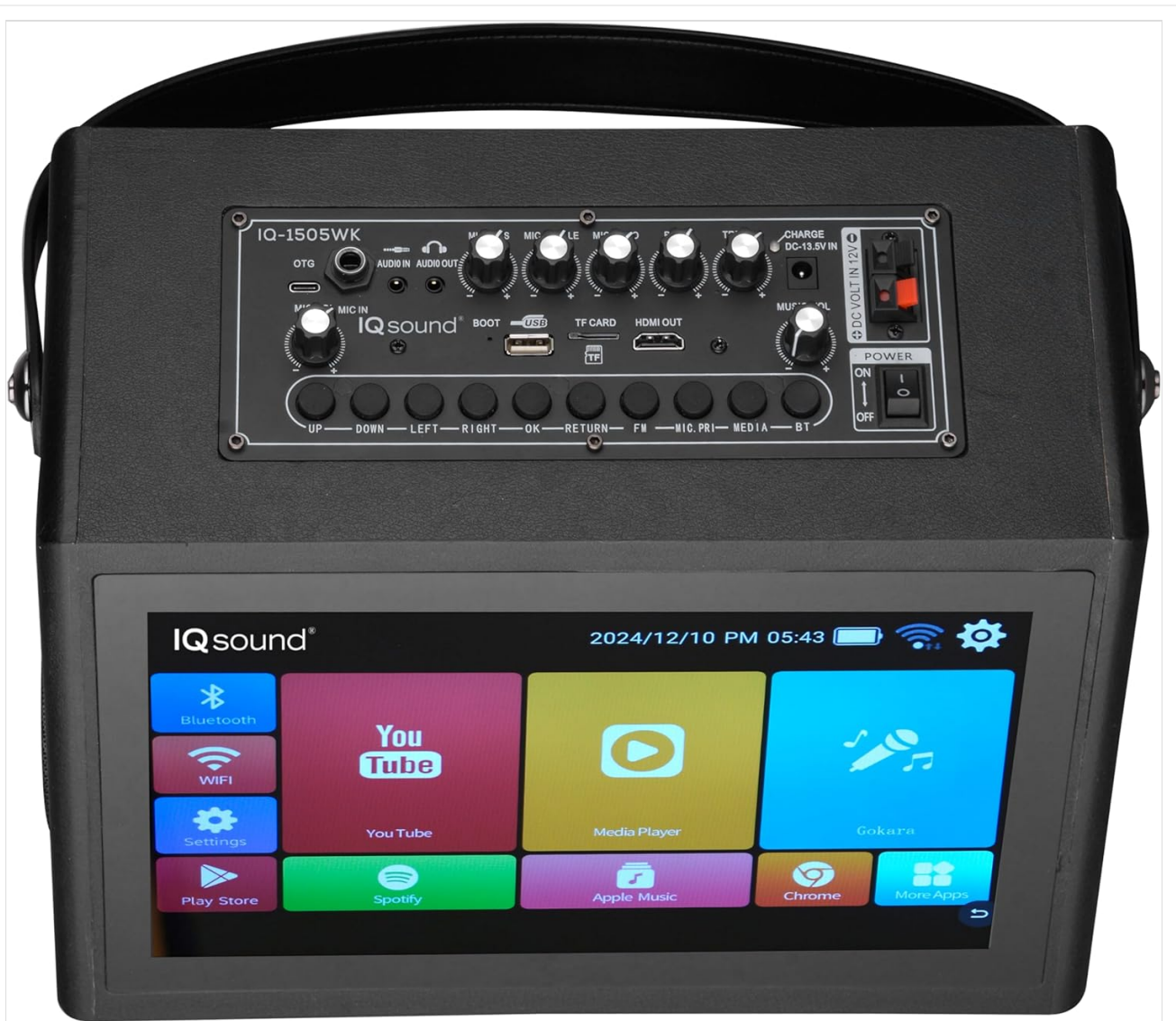
Figure 3: Top Panel Controls. This image provides a clear view of the top control panel. It features various knobs for volume, microphone input, echo, and bass/treble adjustments. Input ports such as MIC IN, AUDIO IN/AUDIO OUT, USB, TF CARD (Micro SD), HDMI OUT, and DC 13.5V IN are clearly labeled. A power switch is also visible.
