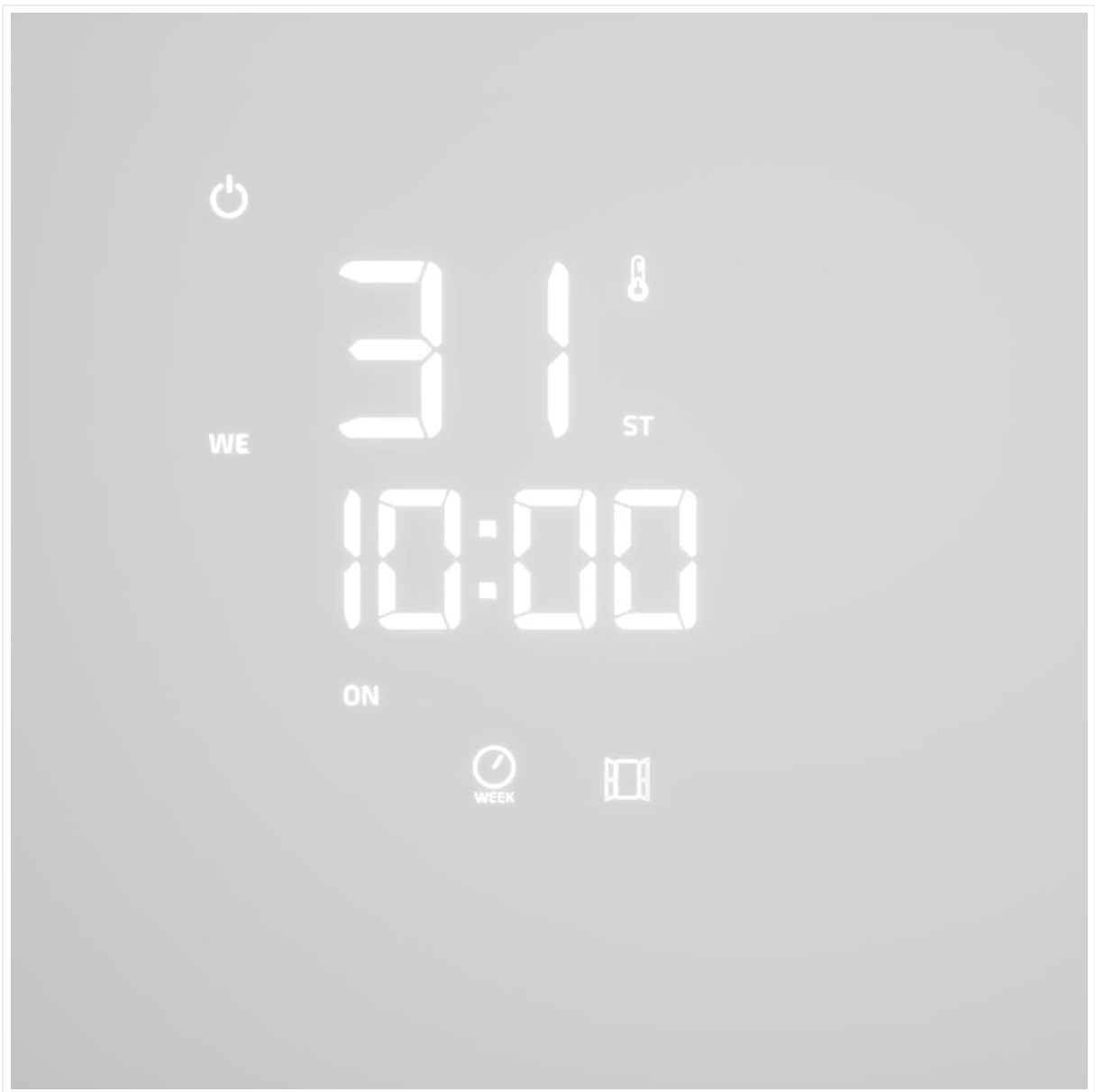
Figure 4.2: A detailed view of the heater's LED display, indicating the current temperature (31 degrees) and time (10:00), along with mode icons.
