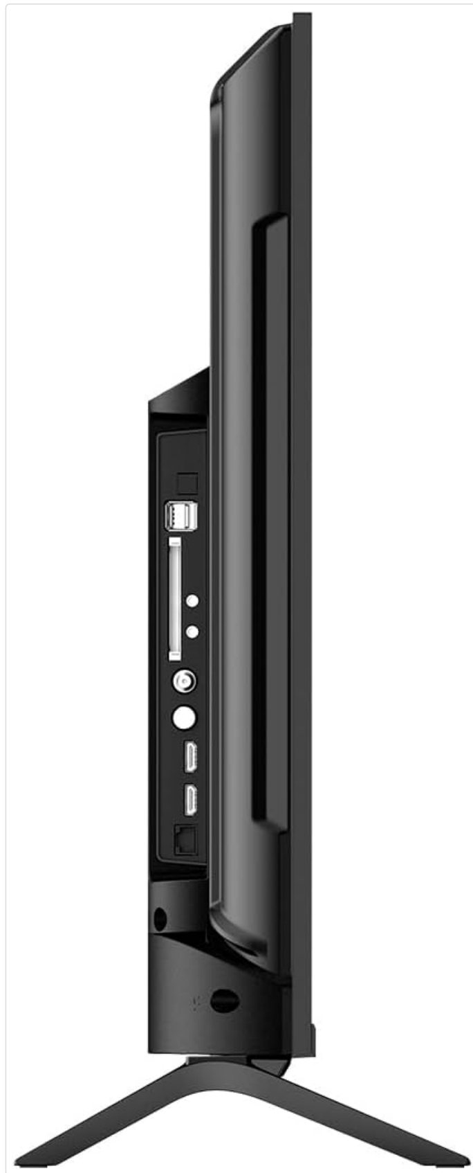
Side view of the Blaupunkt 40FGC5500S 40-inch Full HD Google TV, illustrating the accessible input ports for various devices.
